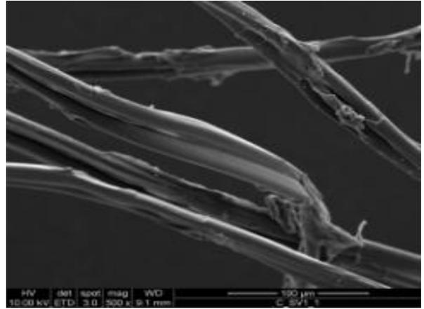
Cocoon silk fibre pre and post treatment with microbial enzymes under Scanning Electron Microscope
